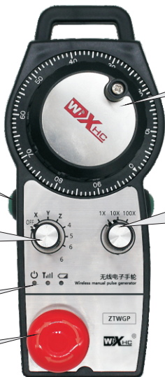
倍率开关, 具有1X, 10X,100X三档调速
